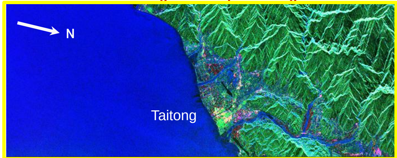
Scattering power decomposition ( Pd , Ps , Pv )
